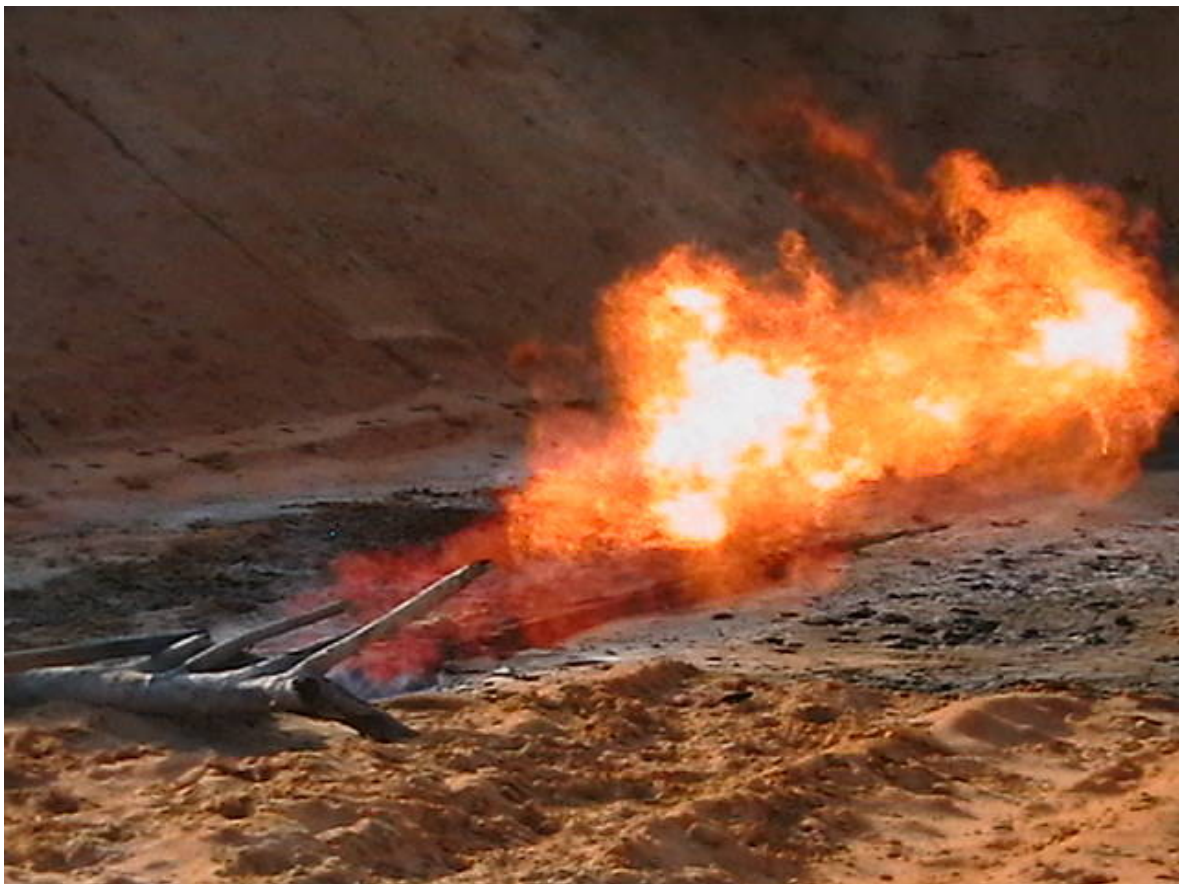
Gas flowing during production testing at Advent's Waggon Creek-1 well in EP386.
